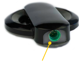
The Nucleus 22 coil has a green connector for the coil cable
